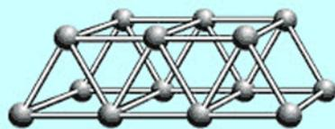
If you want to, you can use your gumdrops and toothpicks to build some strong structures that are made by combining triangles and squares. The pattern on the left is one that's similar to some used in modern bridge design.
