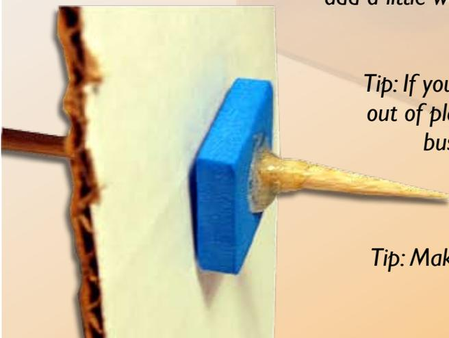
*Tip:* Make sure to glue the bushing to the axle and **NOT** to the frame.
