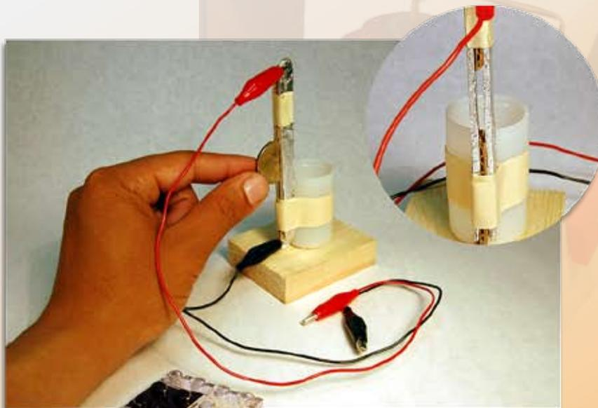
Program a PicoCricket to send power to a LEGO motor when it detects a coin completing the circuit in a coin detector.
